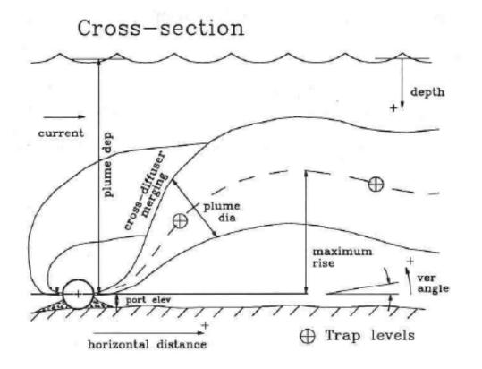
UM3 model (three-dimensional Updated Merge model) of the EPA PLUMES is embedded in the diffuser code;
