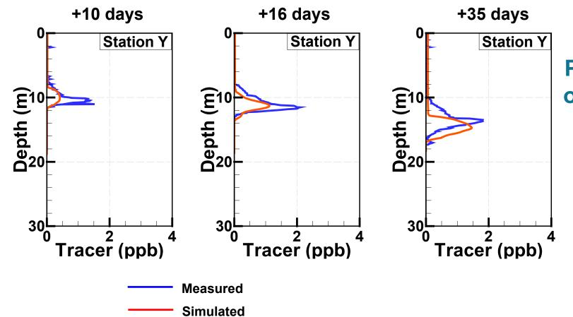
Profiles show visual match of measured and simulated tracer concentrations
