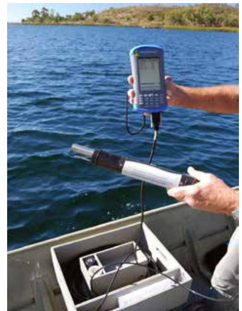
Figure 4. Left, preparation of the Rhodamine WT tracer prior to injection ten meters below the platform. Right, instrument used to measure Rhodamine WT in vertical profiles; the fluorometric sensor can reliably measure Rhodamine WT concentrations to 0.1 ppb.
