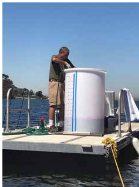
Figure 4. Left, preparation of the Rhodamine WT tracer prior to injection ten meters below the platform. Right, instrument used to measure Rhodamine WT in vertical profiles; the fluorometric sensor can reliably measure Rhodamine WT concentrations to 0.1 ppb.
