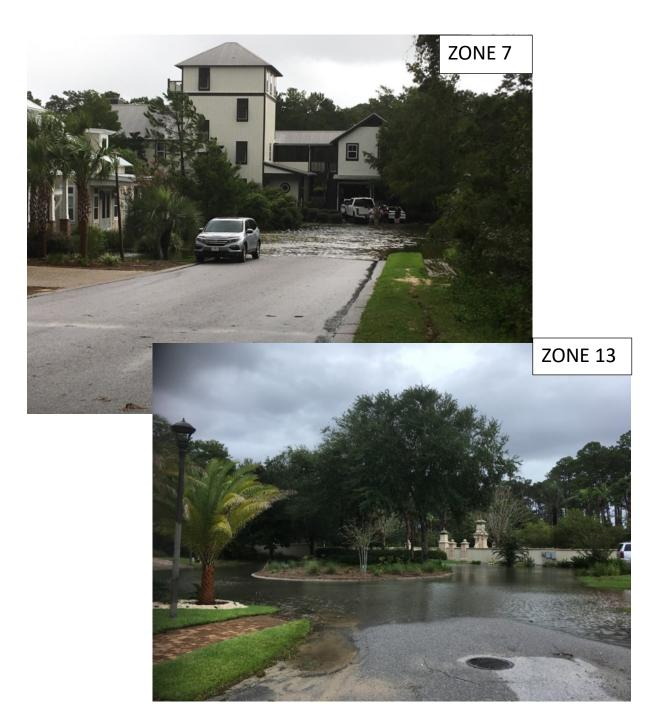
According to the two engineering firms that we met with, the rainfall from Hurricane Sally exceeded the 25-year storm design threshold of our common area storm system and was closer to a 100-year event.
