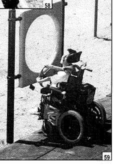
Elevated play components accessed by transfer systems do not require maneuvering or clear floor spaces, since mobility devices are left at ground level.
