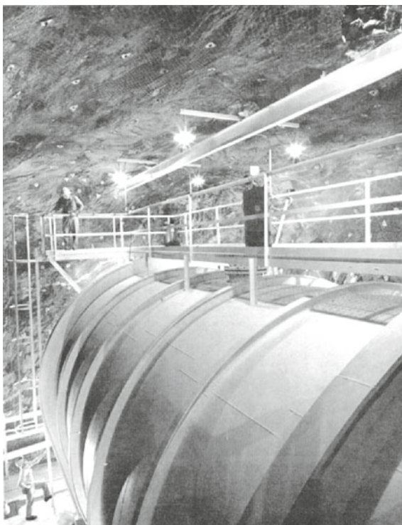
Fig. 5.14 The chlorine experiment one kilometre below the ground in the Homestake Gold Mine in South Dakota, USA. The steel tank contains 400,000 litres of \text{C}_2\text{Cl}_4 . When a neutrino interacts with a chlorine nucleus, a radioactive nucleus of argon is produced. The name of the game was to extract the few argon atoms out of a total of 1030 chlorine atoms in the tank!
