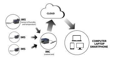
The **IMS** SENSORS measure the temperature and the humidity in the room and send the information to the **IMC**, the GSM COMMUNICATION UNIT.
