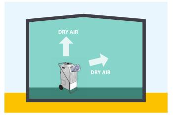
**ROOM DRYING.** With the ACD 137 placed inside the room the dry air is blown around the room. The humidity removed from the air is collected into a tank.
