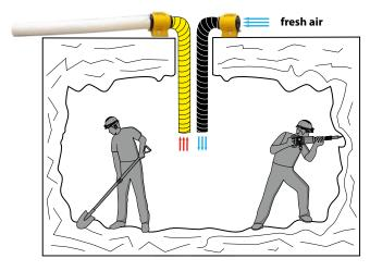
Example: underground works – fresh air is blown in, used air is blown out and filtered.
