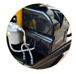
The heater gets the fuel from the tank below but can also be connected to an external tank.
