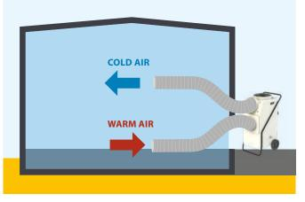
**ROOM COOLING.** The ACD 137 is placed outside a small room. The air is recirculated. The TAC room thermostat is placed inside the room to control the temperature.
