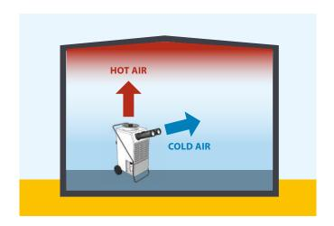
**SPOT COOLING.** Placed into a room the cold air is blown towards the target (for example an electronic device that needs cooling down) and the hot air is blown upwards.
