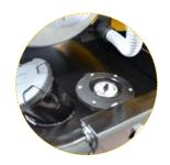
A leakless fuel tank closure and a big fuel level indicator.
