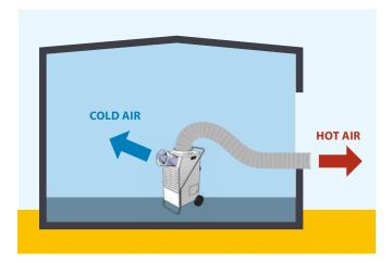
**ROOM COOLING.** The ACD 137 is placed inside a room and the cold air is blown into the room with the hot air ducted outside.
