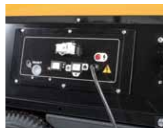
Control panel with thermostat socket (analog or digital)
