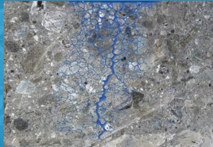
Concrete Cross-Section: Water and chemicals seep into concrete pores and capillaries causing cracks and corrosion.
