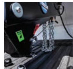
Safety chains with clevis hook and storage on unit
