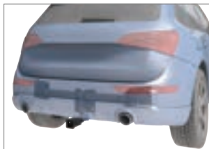
Hidden Hitch® installed with receiver assembly inserted
