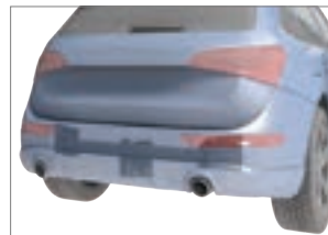
Hidden Hitch® installed with receiver assembly removed
