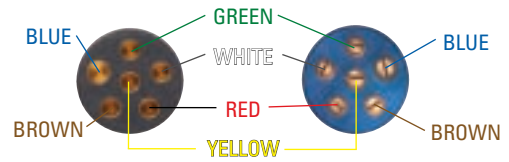
TRAILER END As viewed from core back side where wires are attached with screws.
