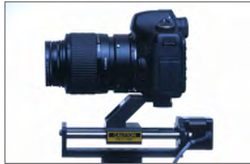
Fig 13 Another useful tool to make focusing easier at large magnification is a macro slide rail.
