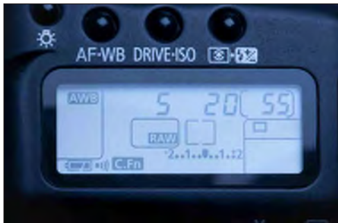
Fig 12 The aperture value should be set to f20 . The exposure time will be adjusted automatically when in AV mode.
