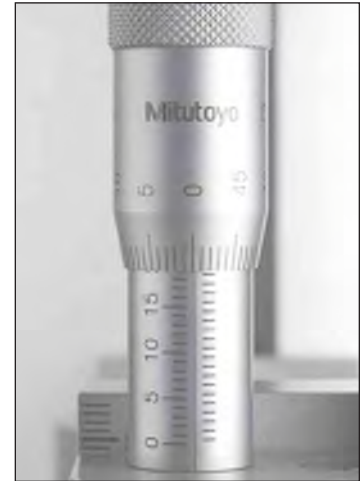
Fig 3 Slice thickness can be controlled by adjusting the micrometer of the support arm of the milling machine.
