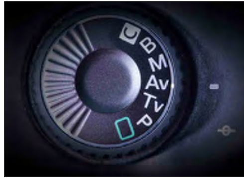
Fig 11 The shooting mode should be set to Aperture Value.
