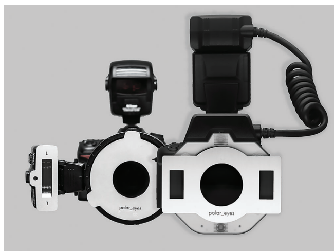
FIGURE 1 The use of cross polarization presents a convenient method to record the appearance of teeth without their specular reflections (gloss) to ensure accurate color measurement. The most straightforward approach to achieving adequate cross polarization is with the use of a ring flash, paired with the appropriate cross polarization filter
