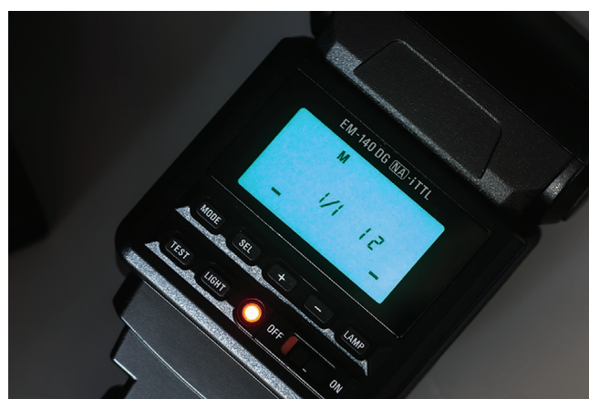
FIGURE 3 For cross polarized photography it is of paramount importance to switch off E-TTL and to use the manual mode instead, with flash intensity set to maximum (1:1) on all channels in order to prevent severely underexposed images
