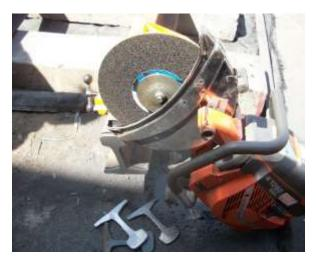
In both bench tests and site trials The Rail Clamp Company **Quantum Superior** Plus 14 Inch Disc Blade managed 5 cuts straight through standard 113lb/UIC54 rail section before requiring the need for replacement. These test results were achieved with the blade fixed to a Husqvarna K1260 Rail Cutting Machine.
