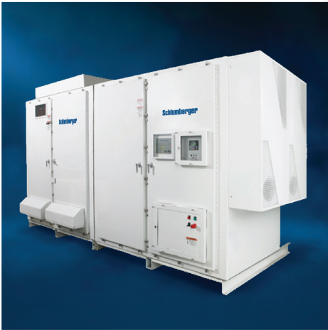
The outdoor MVD, the first of its type in the industry, is designed standard with a visible disconnect switch, precharge circuitry, 36-pulse input and sine wave drive output filter specifically tailored for controlling and protecting high-horsepower ESPs and surface pumps. The outdoor MVD does not require installation in a climate-controlled environment.
