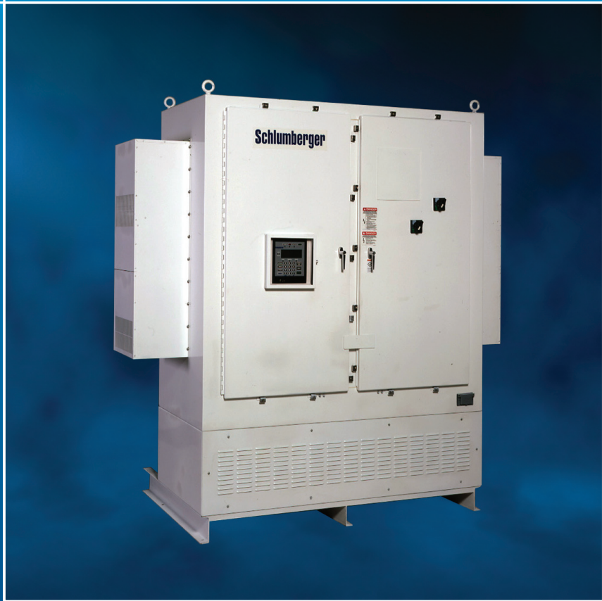
SpeedStar 519 SWD 18-pulse, low-voltage package is designed to minimize supply power harmonic current and voltage distortion, while providing clean power to the downstream device.
