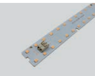
LED Module: 2835LED 28W/1.2M
