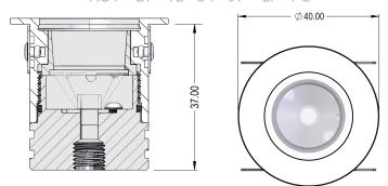
Please allow 10mm for cable gland for IP67 CUT-OUT - 32Ø
