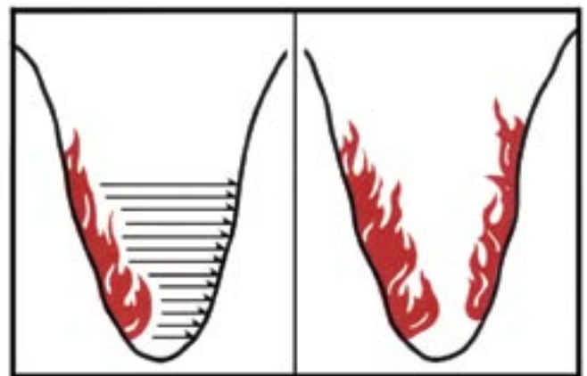
Flashover in V-shaped valley.
