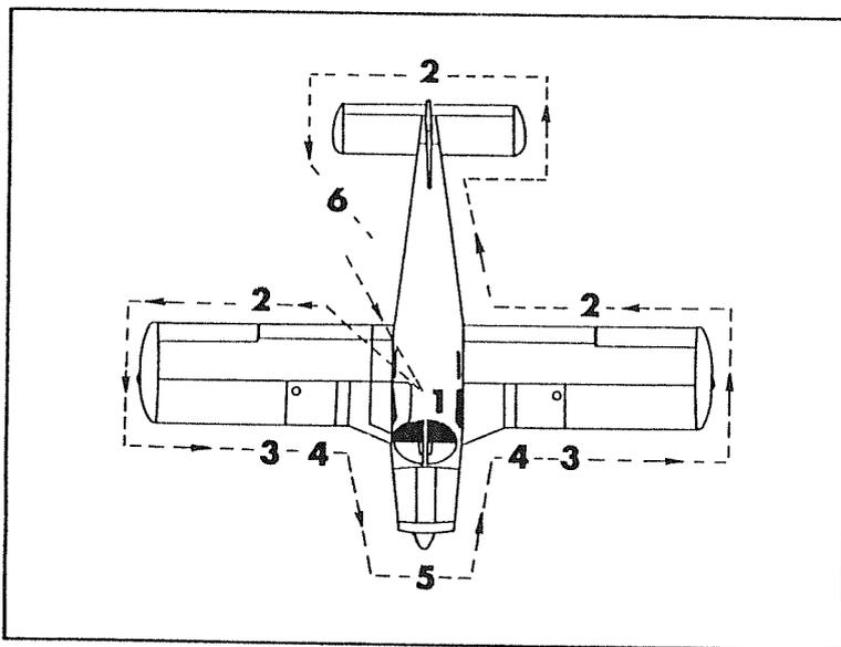
4. a. The landing gear shock struts are properly inflated. (Refer to Section V)
