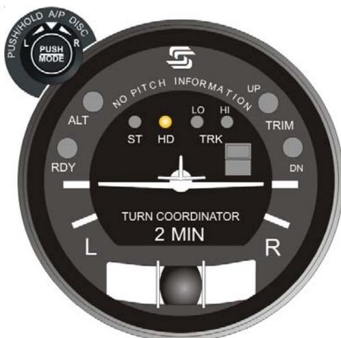
**Fig. 2-22. AP Display, HD Mode Engaged
