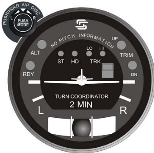
**Fig. 2-11. AP Display, Turn Coordinator Failure (System Thirty)**
