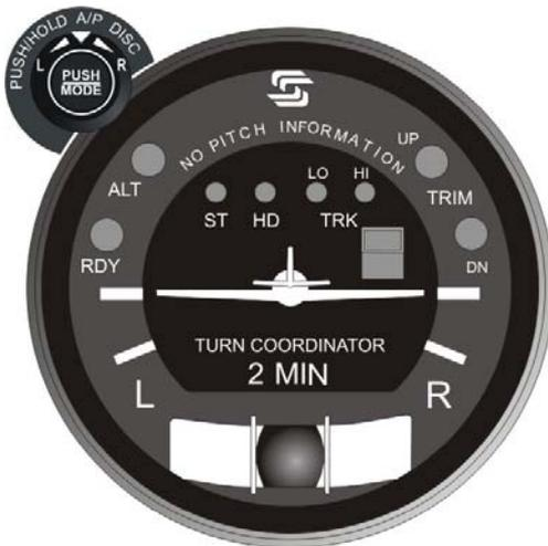
**Fig. 2-2. AP Display, All Lamps Extinguished (System Twenty)**
