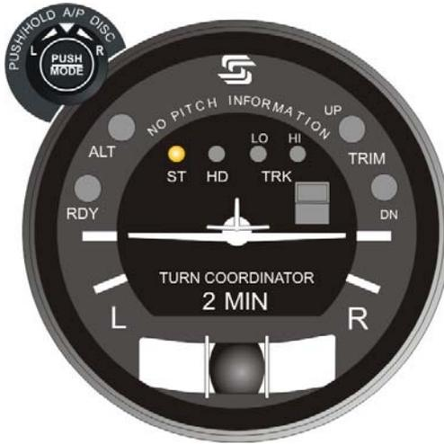
Fig. 3-1. AP Display, ST Mode Engaged
