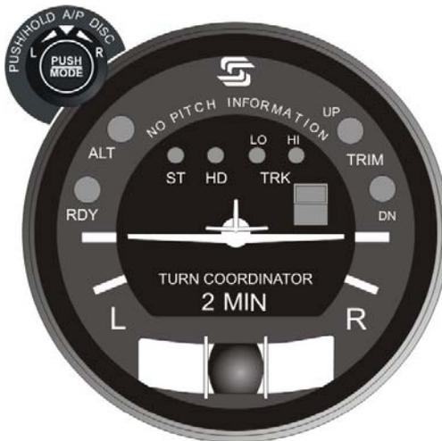
**Fig. 2-4. AP Display, Turn Coordinator Failure (System Twenty)**
