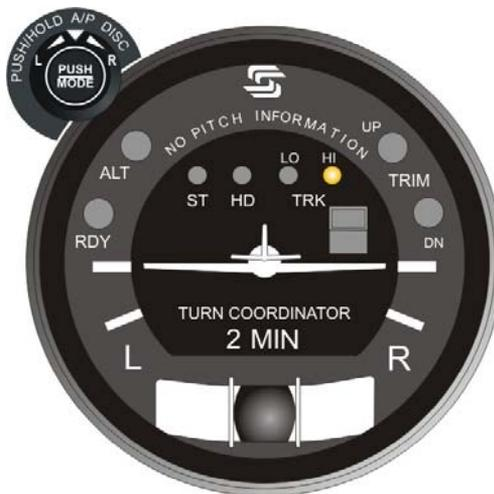
Fig. 3-4. AP Display, HI TRK Mode Engaged
