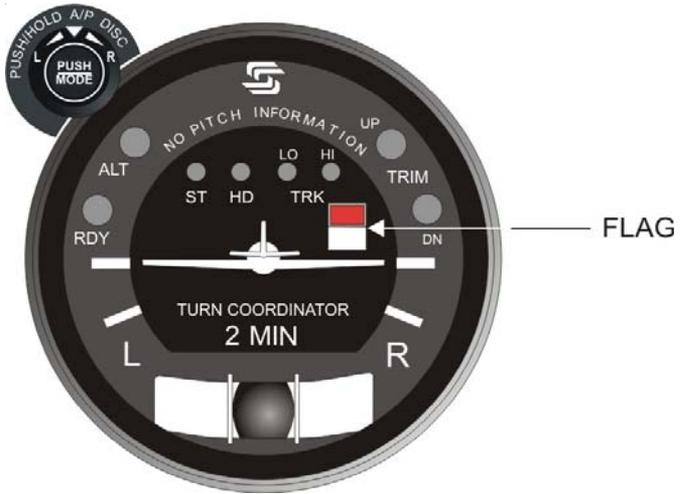
**Fig. 2-5. AP Display, Low Voltage Flag (System Twenty)**
