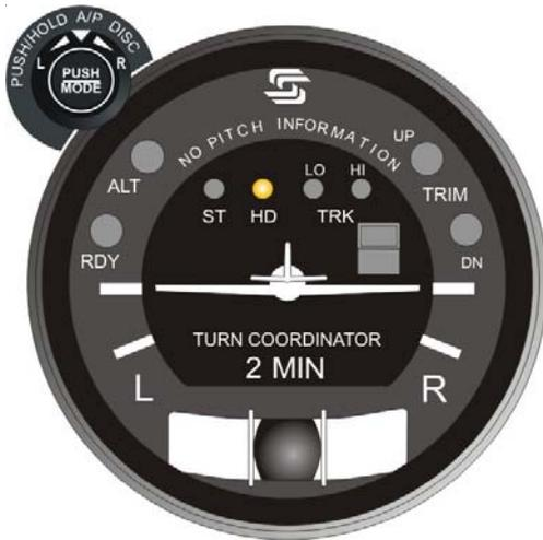
Fig. 3-2. AP Display, HD Mode Engaged
