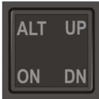
**Fig. 2-16. ALT HOLD ON/OFF Switch Display, ALT ON Lamp Extinguished
