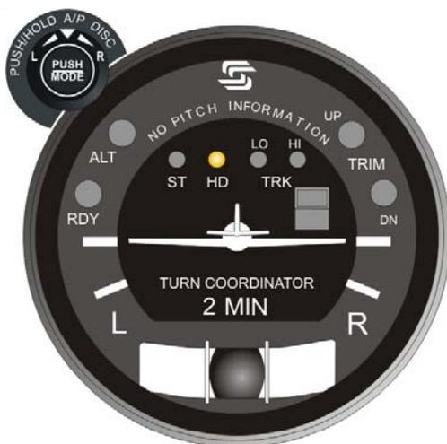
**Fig. 2-18. AP Display, HD Mode Engaged (System Twenty)**
