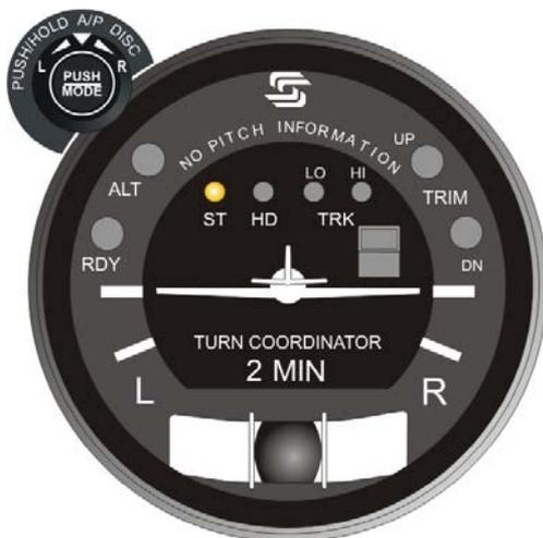
**Fig. 2-17. AP Display, ST Mode Engaged (System Twenty)**
