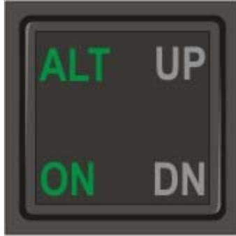
**Fig. 2-15. ALT HOLD ON/OFF Switch Display, DN Lamp Extinguished
