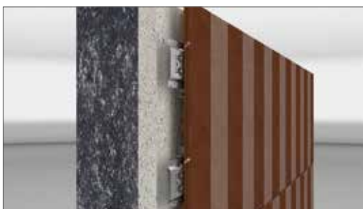
Securing of the position of the panels at the K20 Omega profiles (with securing brackets)
