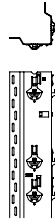
Article 633 Omega profile, external angle* Material: AlMg3 H22 (EN AW-5754), unpainted, for the installation of mitre-cut panels and external angle profiles
