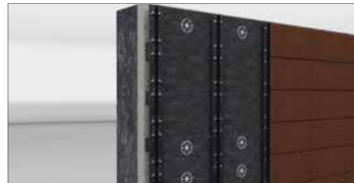
Mount the T-profile with approved fastening means
