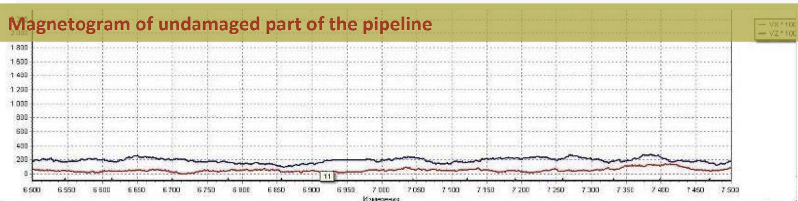
Magnetogram of undamaged part of the pipeline
