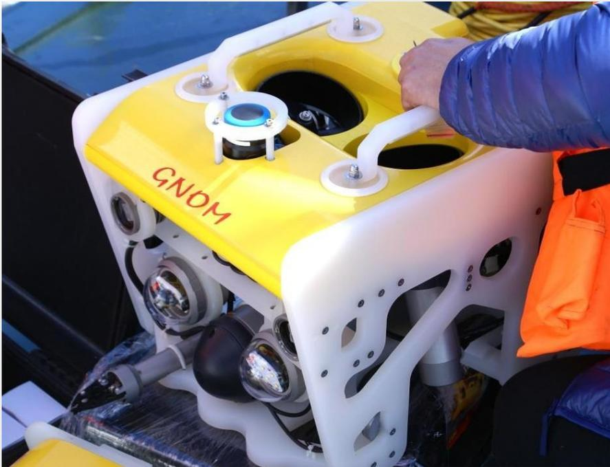
KMD-02GR-Dolphin mounted on SuperGnom ROV and ready for the operation.
