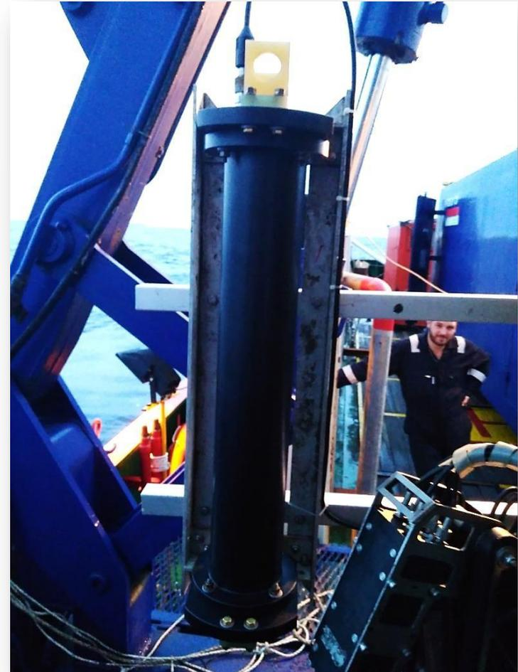
KMD-02R-Barracuda is mounted on an ROV.
