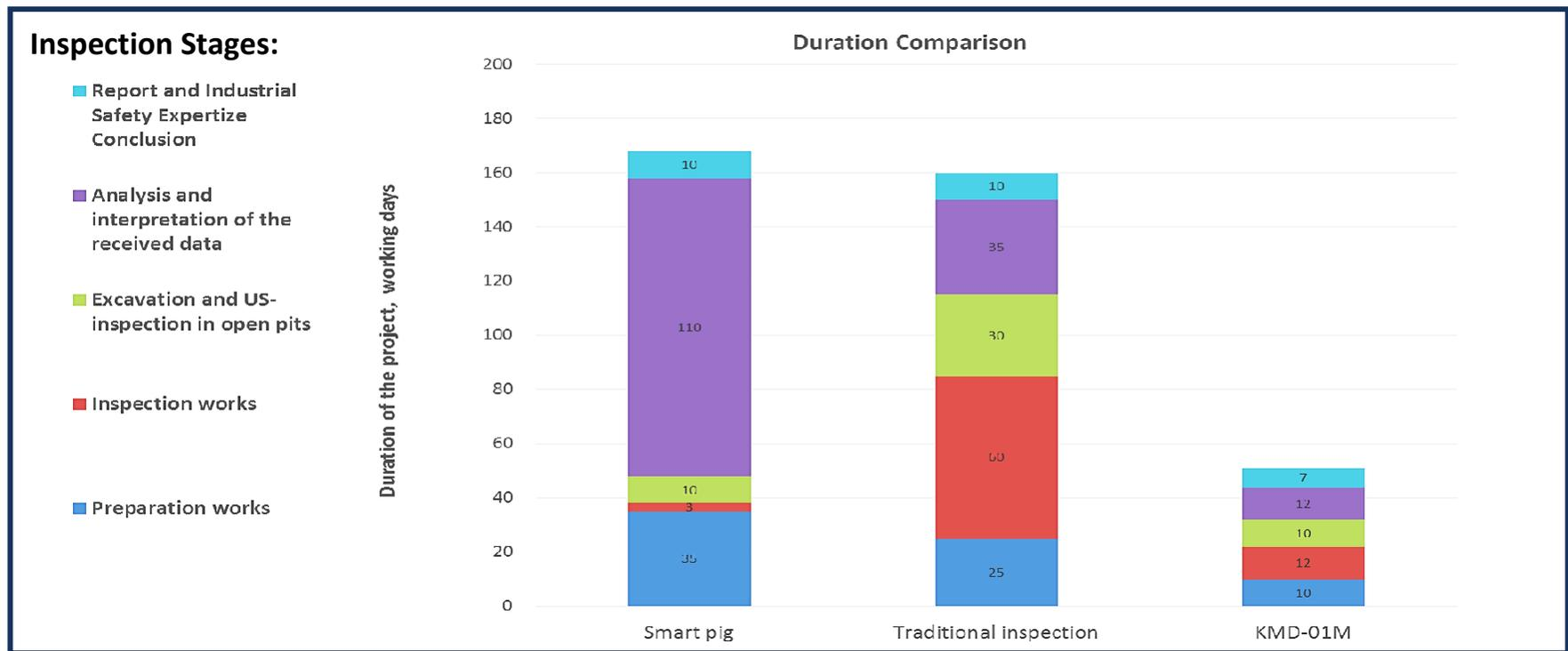
\* Traditional inspection - Ultrasonic and similar contact tests in the pits excavated each 500 m.
