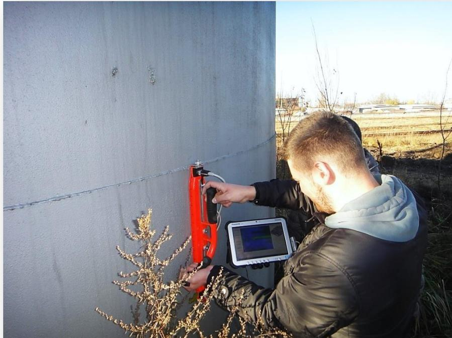
The system allows inspection of tanks even without a pressure.
