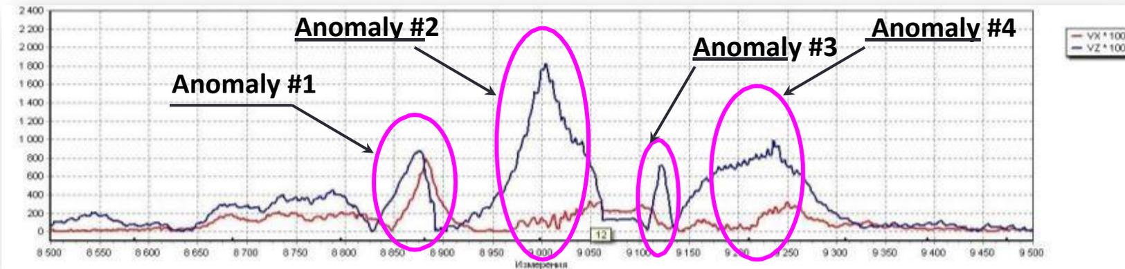
Magnetogram of the damaged sections of the pipeline
