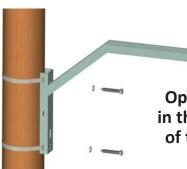
Option 2: Two wood screws in the upper and lower parts of the bracket, plus 2 bands for better reliability
