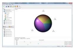
The analyzer has four independent Measurement Points. Each Measurement Point can be set individually to perform four different types of registration without need to change analyzer's configuration.
