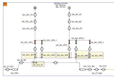
flow and pressure data to provide a highly-accurate calculation of the hydraulics and composition of products in a pipeline in real-time, while the Tuning Assistant keeps the model as close to reality as possible. Atmos Batch is a module of Atmos SIM and uses the same schematic as the pipeline model, Atmos SIM leak detection, and Atmos Pig.
