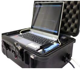
remote access using mobile broadband modems connected to the netbook computer of the data logger kit (provided there is mobile broadband coverage).
