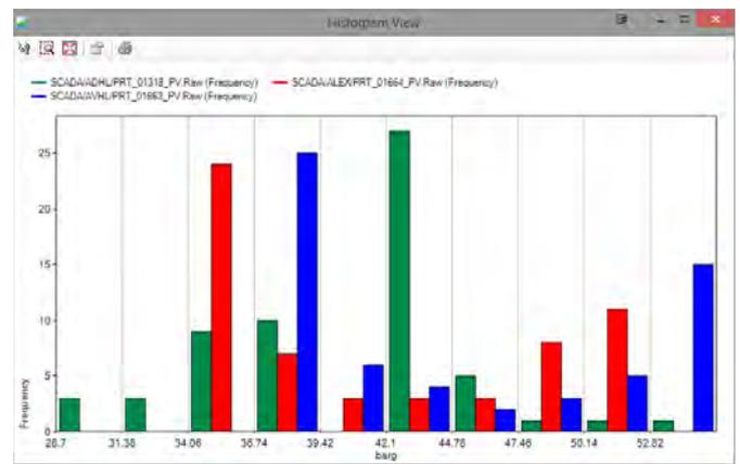
Figure 3. The fully customizable histogram option gives the operator the distribution of values for a set of meters
