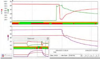
Figure 1: Trend with overview screen and zoomed into a smaller time range, also showing discrete values as an enumeration bar
