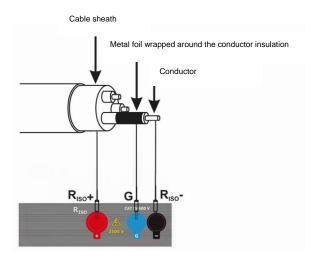
The same shall apply when measuring the resistance between two conductors of the cable, attaching to  ${\bf G}$  terminal other conductors that do not take part in the measurement.
