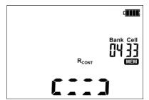
The cell is partially occupied by a different type of result to be entered - symbols of the saved values are displayed.
