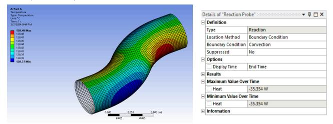
The outside surface of the metal pipe had a max temperature of 128.5 deg C and the overall heat lost from the convection at the outermost surface was -35.4 W.
