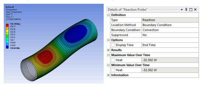
The outside surface of the metal pipe had a max temperature of 130.8 deg C and the overall heat lost from the convection at the outermost surface was -32.3 W. The heat loss was lower than Part A because the convection coefficient of the surface was lower (3.4 vs 3.8 W/m²-C) meaning less heat was transferred to the outside air. The equivalent convection coefficient was derived from the equations below using the metal pipe/foam thickness and material properties.
