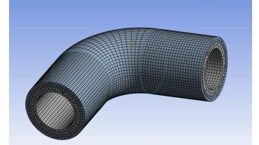
Three meshes were generated for Part B with default settings and element sizes of 5mm, 20mm, and 100mm respectively. There were small observed differences between results, thereby indicating that the mesh is converged. 5mm shown on the next page.
