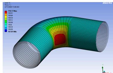
The outside surface of the insulation had a max temperature of 110 deg C and the critical radius was determined to be 54mm using r = k/h. This result was empirically verified by using radii of 53mm and 55mm to verify that the heat loss was indeed lower. Heat loss at 54mm was -40.153 W while it was -40.149 W at 53mm and -40.133 W at 55mm, thereby confirming 54mm is indeed the correct critical radius.
