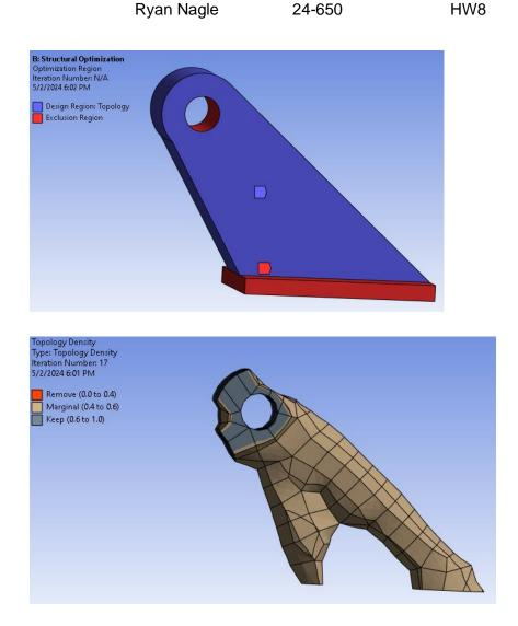
From this optimization, Fusion360 was used to create a shape similar in topology using multiple elliptical cross-sections and the loft feature. From there, the cylindrical connection point was extruded using the dimensions from the A8geom file. Overall, it took 6 iterations of modifying the shape to achieve a desirable result. Full converged results are below.
