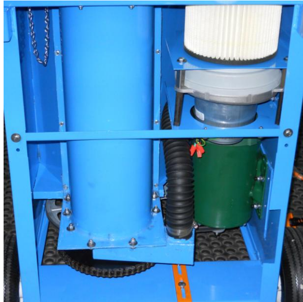
Airlock, blower support bar, and blower connector hose Figure 8
