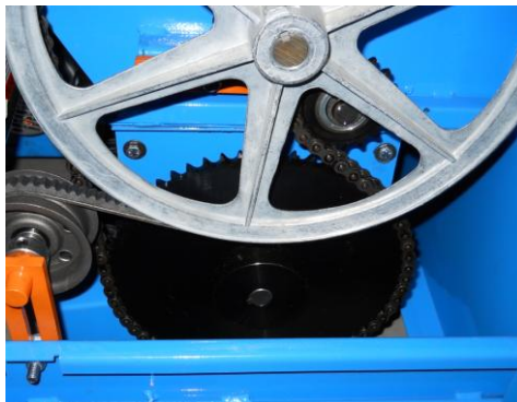
Belt tensioner, airlock sprocket, chain tensioner, and large pulley Figure 7
