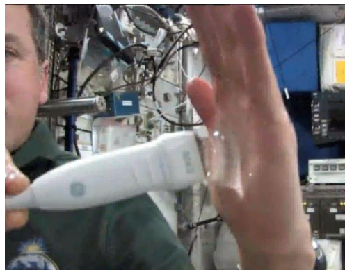
Water as coupling medium in microgravity
