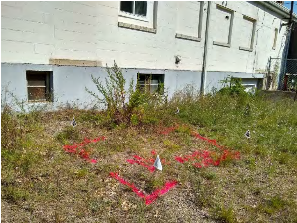
GEC Project No. 1936-0030. July 30, 2020. 2210 Providence Highway, Walpole, MA. Delineation of the UST identified during the geophysical survey.
