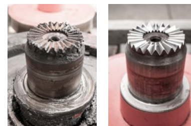
Example of gear profile reconditioning
