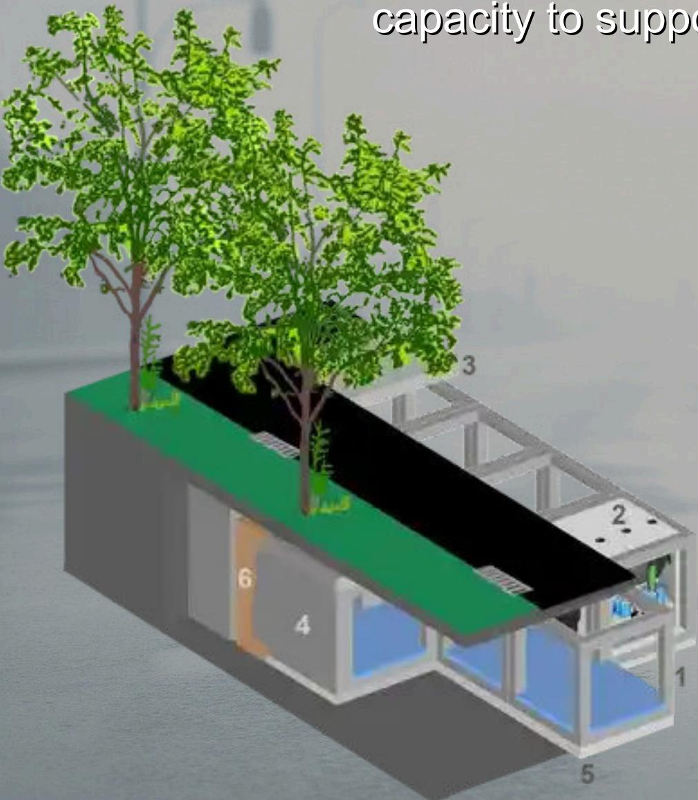
1. Core of the system: A massive, hollow, load-bearing concrete module (2.5 m cube) with an impressive capacity to support up to 792 tonnes.
