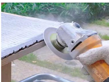
1. Grinding to make 45° chamfer
