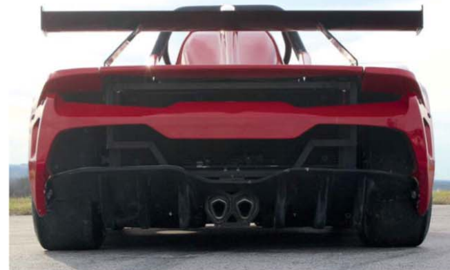
The twin exhausts connect to a Suzuki GSX-S 1000cc powerplant. Aero includes a wing and a modest diffuser at the rear
