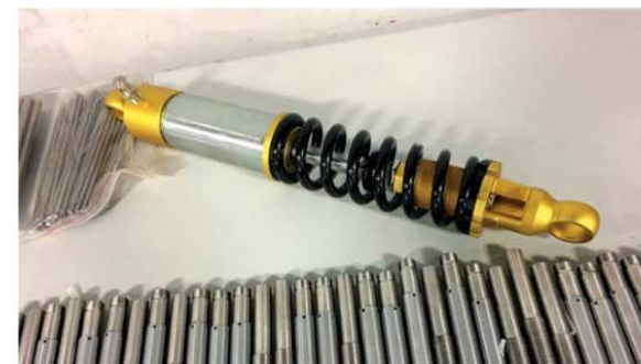
Dampers are of a mono-tube design with nitrogen charged piston. Compression and rebound can be adjusted
