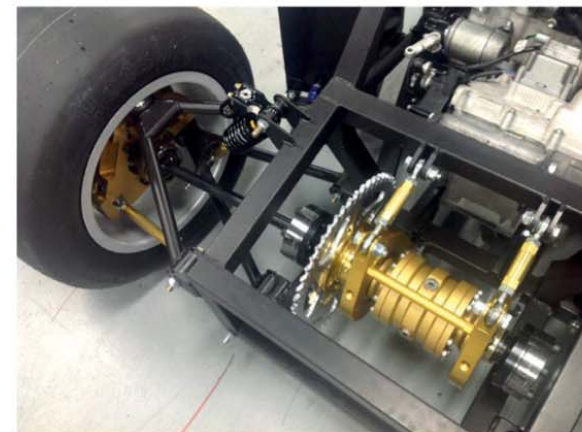
The plate type limited slip differential is just one of many components that Rush has manufactured in-house
