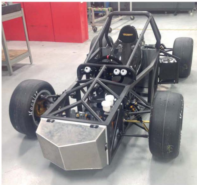
The chassis is made with square tubing, which helps make the build process cost effective. Note the sturdy double roll bar
