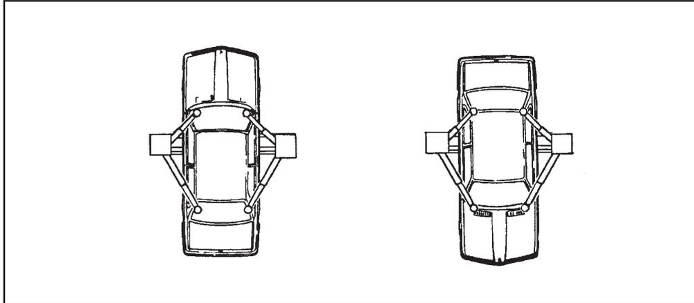
Fig.15 Correctly loaded vehicle
