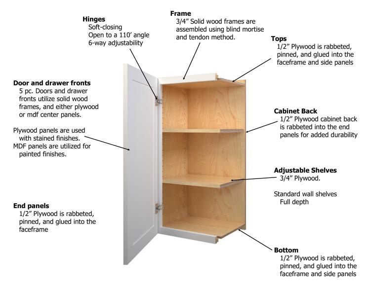
**Finished end panels** are 1/2" plywood with clear natural veneer on the inside and finished veneer on the exposed side.
