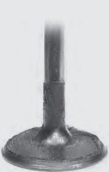
Intake valve after P.i. treatment
