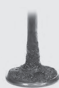
Intake valve before P.i. treatment
