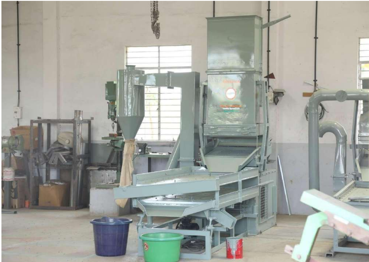
“VISHWA” Pre cleaner with Cyclone Separator
