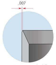
Wagner 007's .007" support bevel allows for reduced wall thickness, use of large springs when needed, and provides straight, accurate cuts with reduced pressure.
