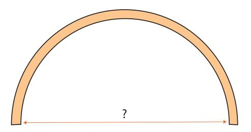
To measure rotary die board inside diameter.
