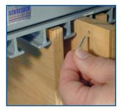
■ Dies are suspended by 3/16" dia. x 1-5/8" long pins, holes can be lasered or routed into dies, or drilled to accommodate.
