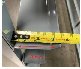
Extra-wide Phase 3 rails provide a secure and strudy platform to safely support dies.
