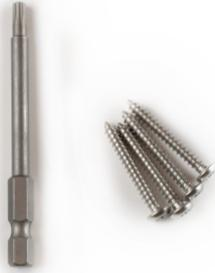
After making all the necessary connections, use the 4 supplied Torx® screws and supplied Torx driver to secure the unit to the wall. It is recommended that you predrill the holes using a 3/32" (2.5mm) bit. Use care to keep the tip of the driver from slipping out of the screw. Use of other screw types could lead to damage of the MS-21 if the driver slips out.
