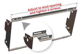
Place frame between studs and secure using the three 1-inch (25mm) screws. While there are 4 holes, the screw where the power supply unit (PSU) will be installed is omitted.
