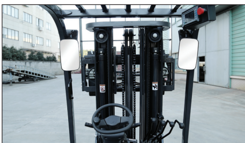
Wide view mast offers good driving vision.
