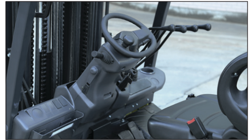
Adjustable steering column according to operator's preference to reduce fatigue.
