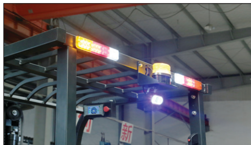
Blue spot light: reminding pedestrians when reversing.
