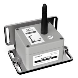
The accelerometer measures the acceleration and temperature of the exact point where it is installed in relation to the structure. It is possible to measure the vibration frequencies and carry out a modal study of the structure. All accelerometers can be perfectly synchronized with each other. Battery power supply and LoRaWAN wireless transmission. The acquisition modes can be set by the user via the web interface provided in the service.
